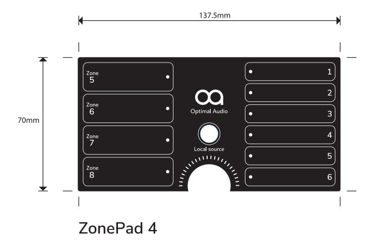
This template is setup for 1 colour print and is shown at 1:1 scale to be inserted into a ZonePad 4 face panel. Please ensure that printing output is at 100%, with dimensions of 137.5mm width and 70mm height. Suitable for printing on an A4 desktop printer or use as a template for commercial printing. A guideline template for die-cutting is on Page 2 of this document.
